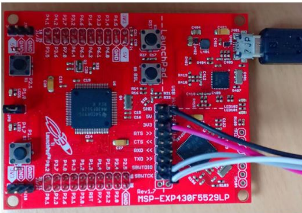
Fig. 7 MSP-EXP430F5529LP for Data Processing
