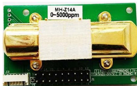
Figure 18 CO 2 sensing module (MH-Z14A)
