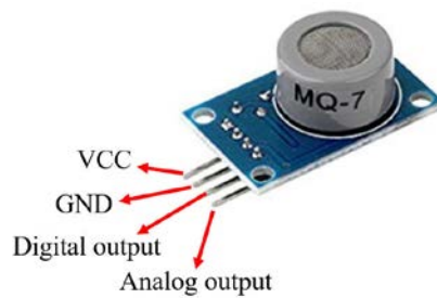
Figure 17 CO sensor module
