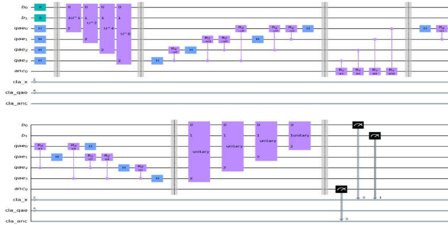
a General HHL algorithm implementation architecture algorithm quantum circuit diagram
