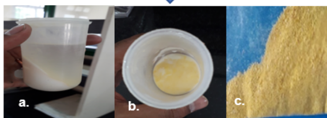
a. & b. Centrifugal separation of starch and gluten slurry c. Dried Gluten
