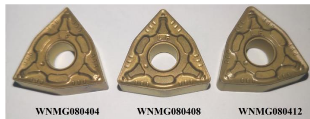
Fig. 4. Three turning tools with different nose radius
