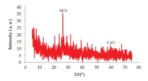
**Figure 3**XRD plot of 4.75 mm size passing sample C
