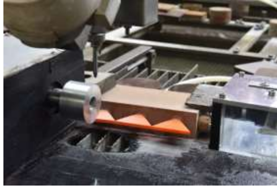
Fig. 3. A specimen placed on the lathe, air blowing system and black polymeric layer on the grid
