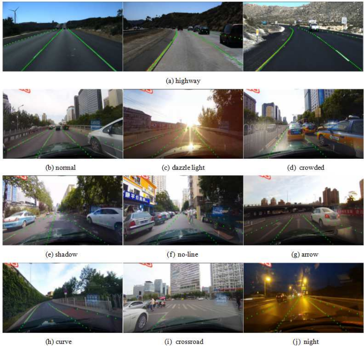
Fig. 2 Visualization of lane detection results. The first row are the results on TuSimple dataset, and the rest are on CULane dataset.
