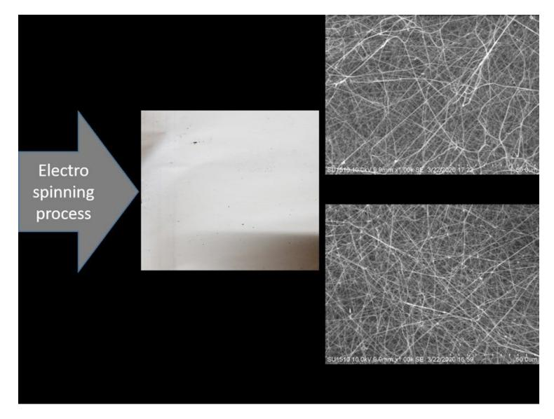
Morphology of electrospun PVA-licorice (a) natural image of membrane (b) SEM image at 10.0 kV, x1.00 k of front site view (c) SEM image at 10.0 kV, x1.00 k of back site view
