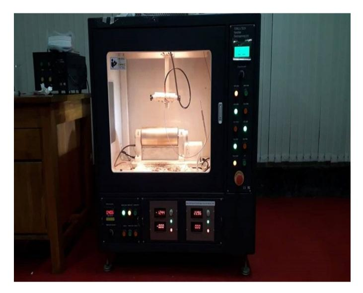
Electro-spinning machine for preparation of membrane
