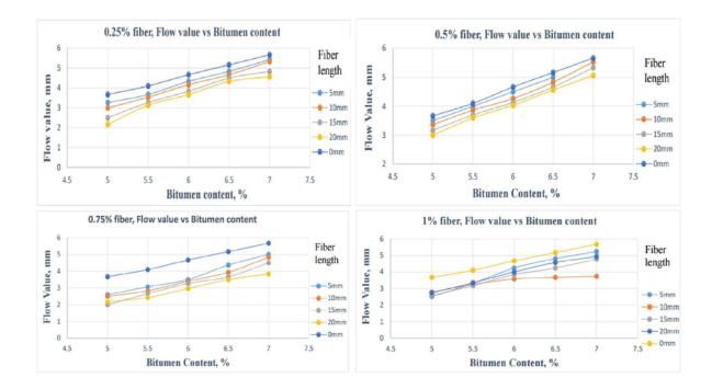
Various amount of fibers present effect on the flow value and bitumen content according to length
