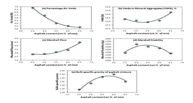
Flexibility of plastic waste materials application in pavement at the different parameters analysis
