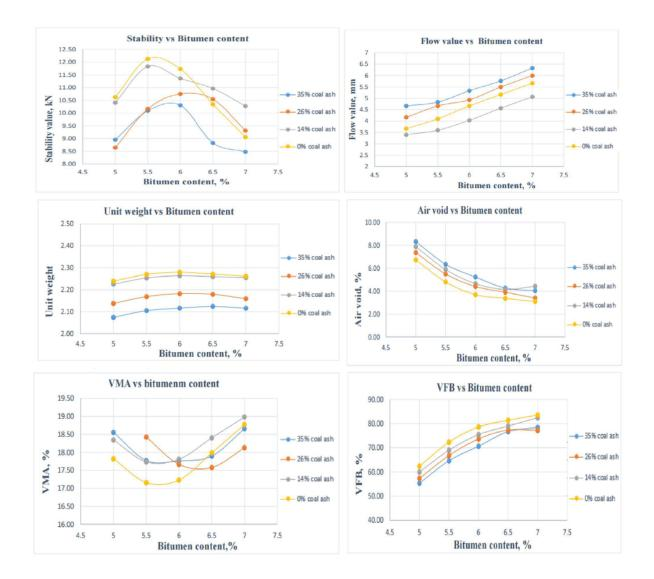
Marshall Stability of bitumen at the flow rate, stability, unit weight and air-void ration
