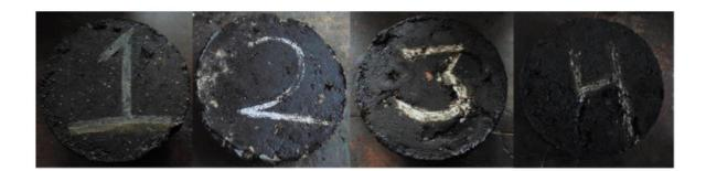
Marshall Specimen with plastic and rubber and bitumen binder (tertiary mix)
