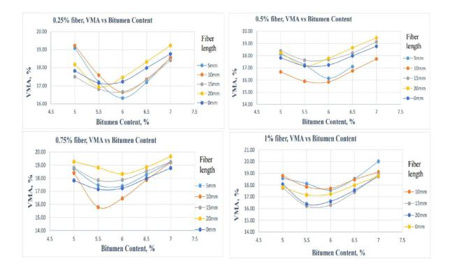
Different percentages of fibers length at VMA vs Bitumen contents
