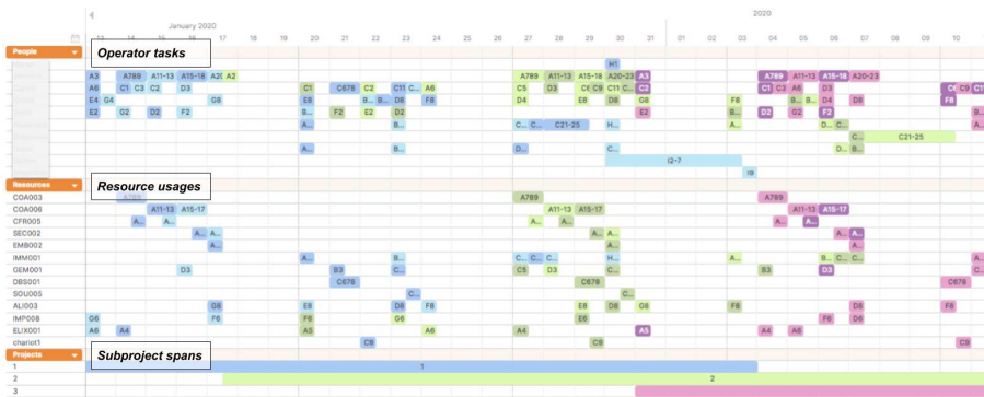
Fig. 7 A possible optimized solution to the problem described by the model depicted in Fig. 6 when three production campaigns are scheduled in parallel. The visualization includes the operators’ task sequences as well as the resource (machines) usages. We see how the campaigns overlap at the bottom with the blue, green and purple bars: each denotes a campaign.
