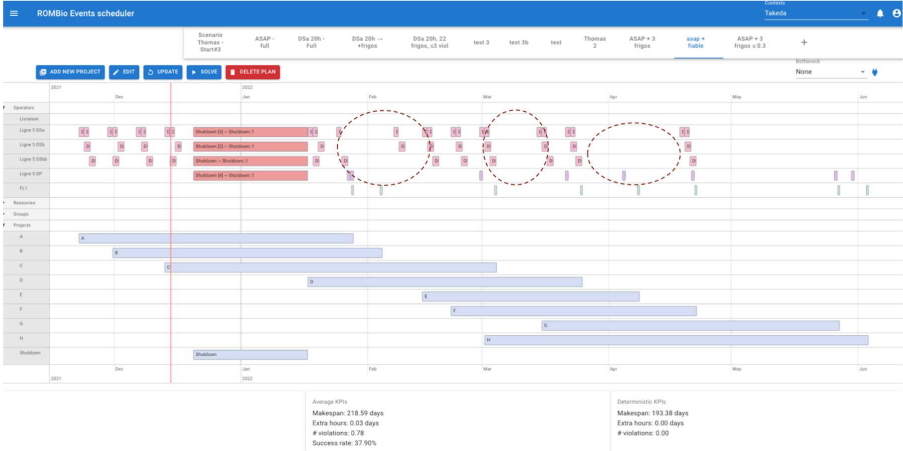
Fig. 13 When asking the system to orient the computation in order to obtain more reliable schedules ( i.e. with higher success probability), the fridge emplacements bottleneck is compensated by introducing slack times (dotted circles).
