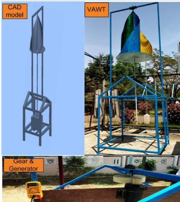
Fig. 3 IWT Practical model with gear and PMDC generator
