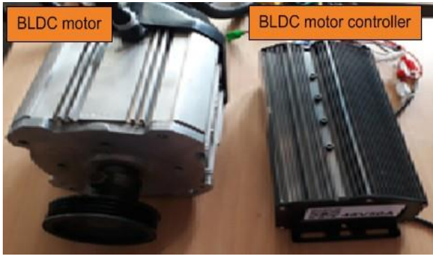
Fig. 5 BLDC Motor with PWM controller
