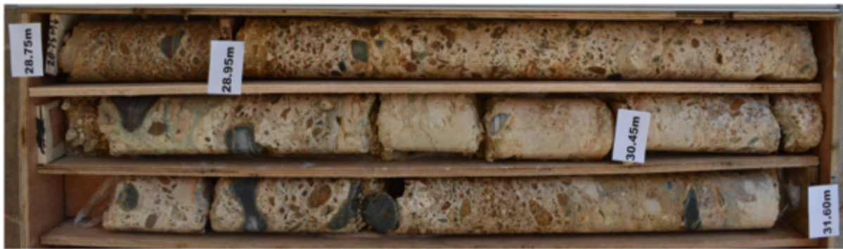
6a 28 to 30m below ground level – Weak to medium strong Conglomerate near the top of barrette
