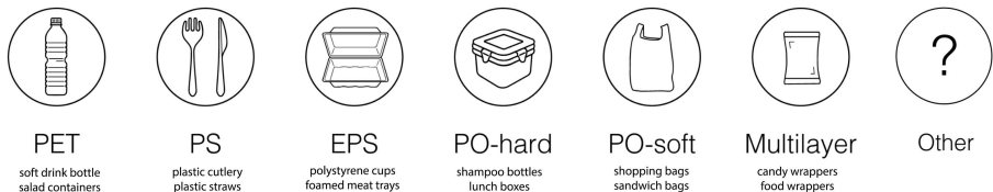
Fig. 2 Categories used for visual counting in this research, with examples of characteristic items for these classes. The 'Other' category contains all anthropogenic litter outside of the six polymer-based classes. Adopted from Tasseron et al. [37].
