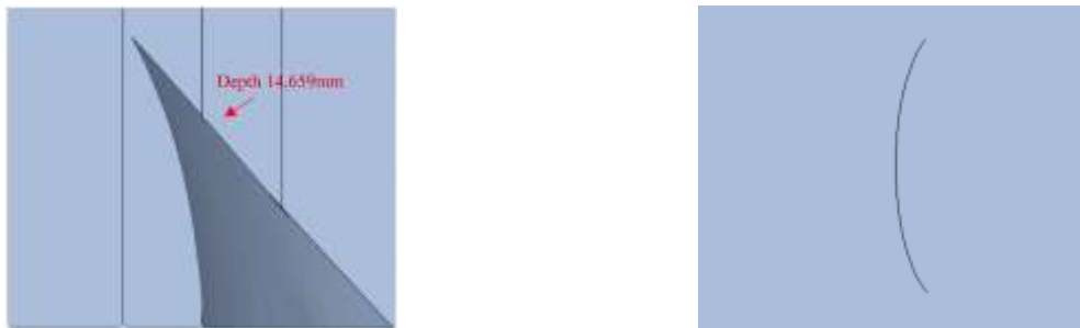
Fig.22 Crack shape simulation in Step 30
