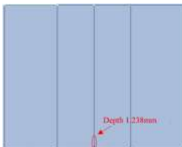
(a) Side view of the crack
