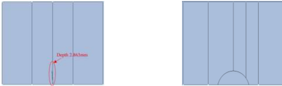
(a) Side view of the crack
