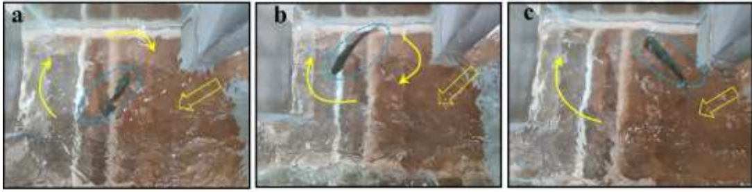
Fig. 10 Q^*=0.261 Fish migration experiment under Q^*=0.261 flow conditions. (Arrows indicate the direction of vortex water flow and vortex)
