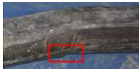
(c) Buckling deformation near supports
