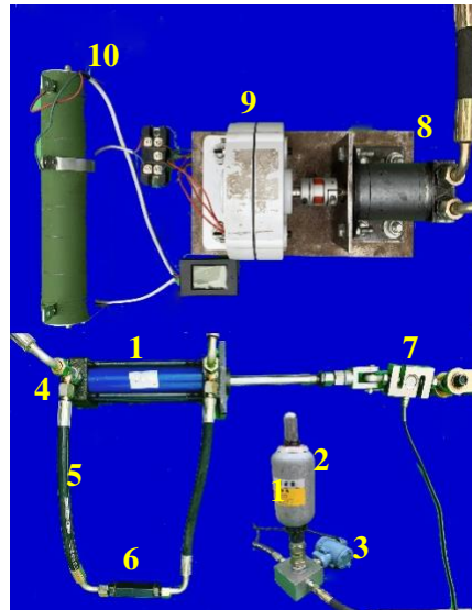
Figure 6. Prototype of Hydraulic Regenerative shock Absorber (1) Hydraulic cylinder (2) Accumulator (3) Pressure Transducer (4, 6) Hydraulic Rectifier (5) Hose (7) Force Transducer (8) Hydraulic Motor (9) Three Phase alternator (10) Sliding Rheostat
