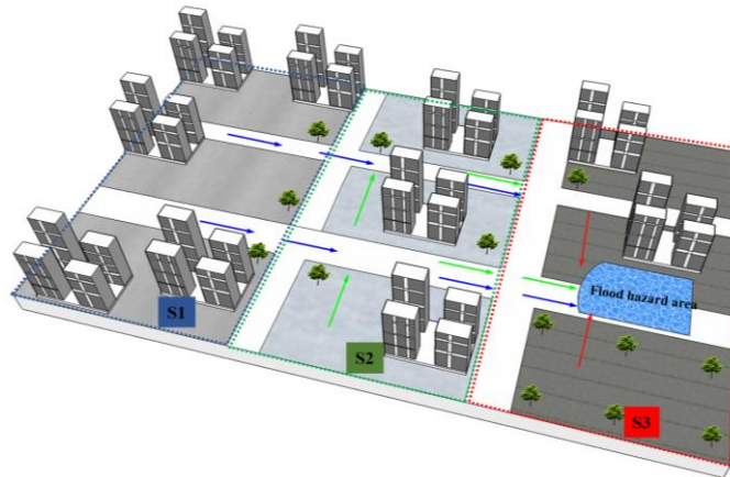
203 204 Fig. 2 Schematic diagram of the runoff source tracking process in urban watershed
