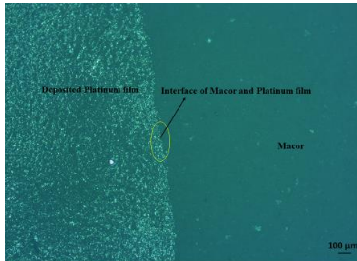
Fig.5: Interface region between Macor and deposited Platinum film
