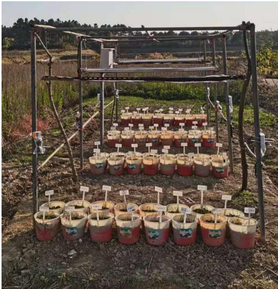
548 Fig. 1 System structure of Free Air Temperature Increased (FATI) in winter wheat field.
