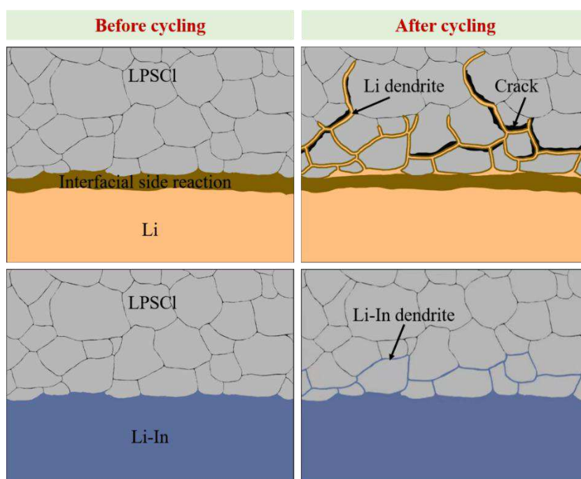
7 8 Figure 7. Schematic diagram of Li-LPSCl and LiIn-LPSCl interface evolution in cells before and 9 after cycling.
