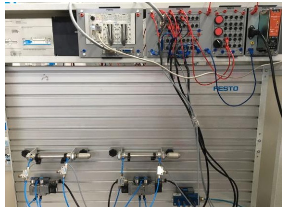
Fig. 43. Circuit designed with the PLC.
