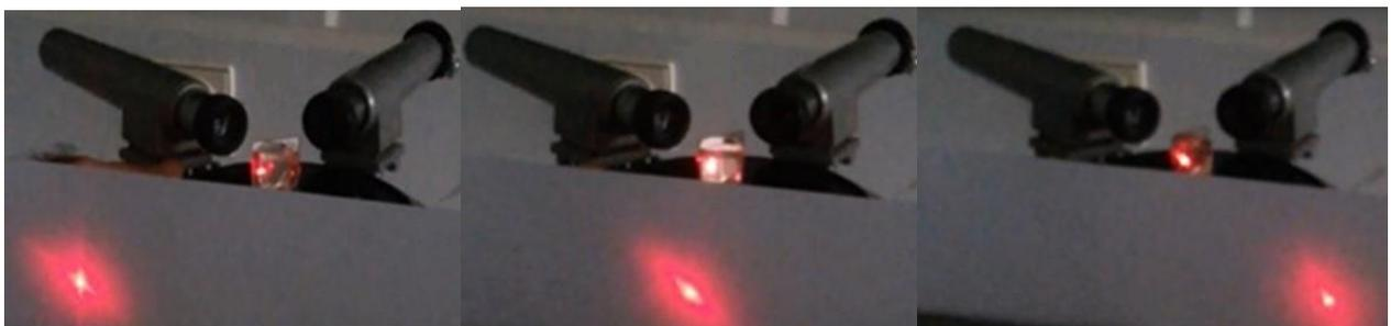
**Fig.7.** Three different displays of S-polarization light intensity reflected on the screen for silver thin film deposited on microscope slide. The optical calibrated turntable rotates from a low angle ( $\theta$ ) to more (from left to right).
