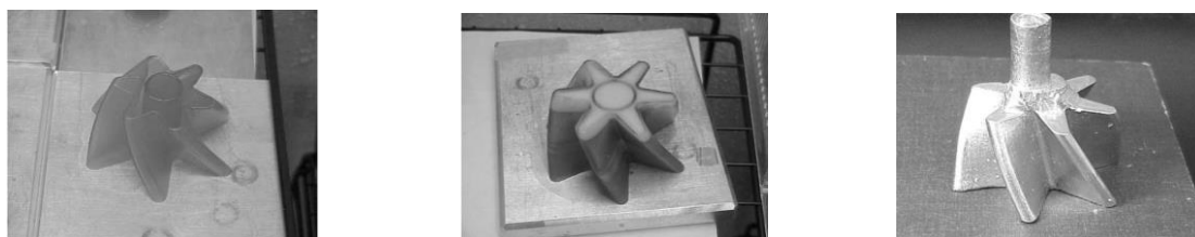
(a) 3D Printed Ice boundary (b) Block of Ice as a Pattern (c) Cast Part
