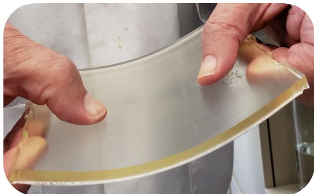
Fig. 7 The sample of epoxy resin prepared from ESO with BCF
