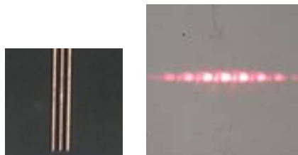
Figure 2.15 Triple slit and its interference pattern
