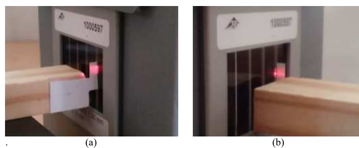
Figure 4.4 Experiments with Shield Contacting Double Slit
