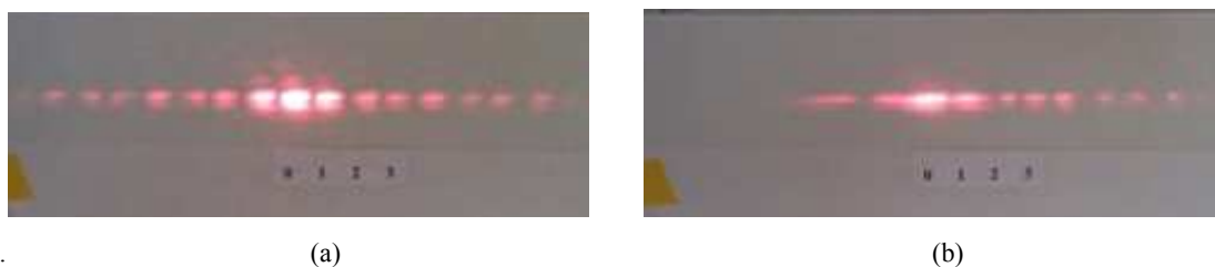
Figure 4.11 Interference pattern of double slit experiment
