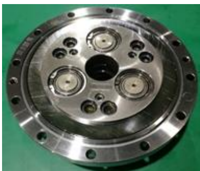
Fig.14 RV reducer prototype
