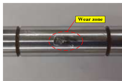
Fig. 2 Extrusion wear diagram of bar surface
