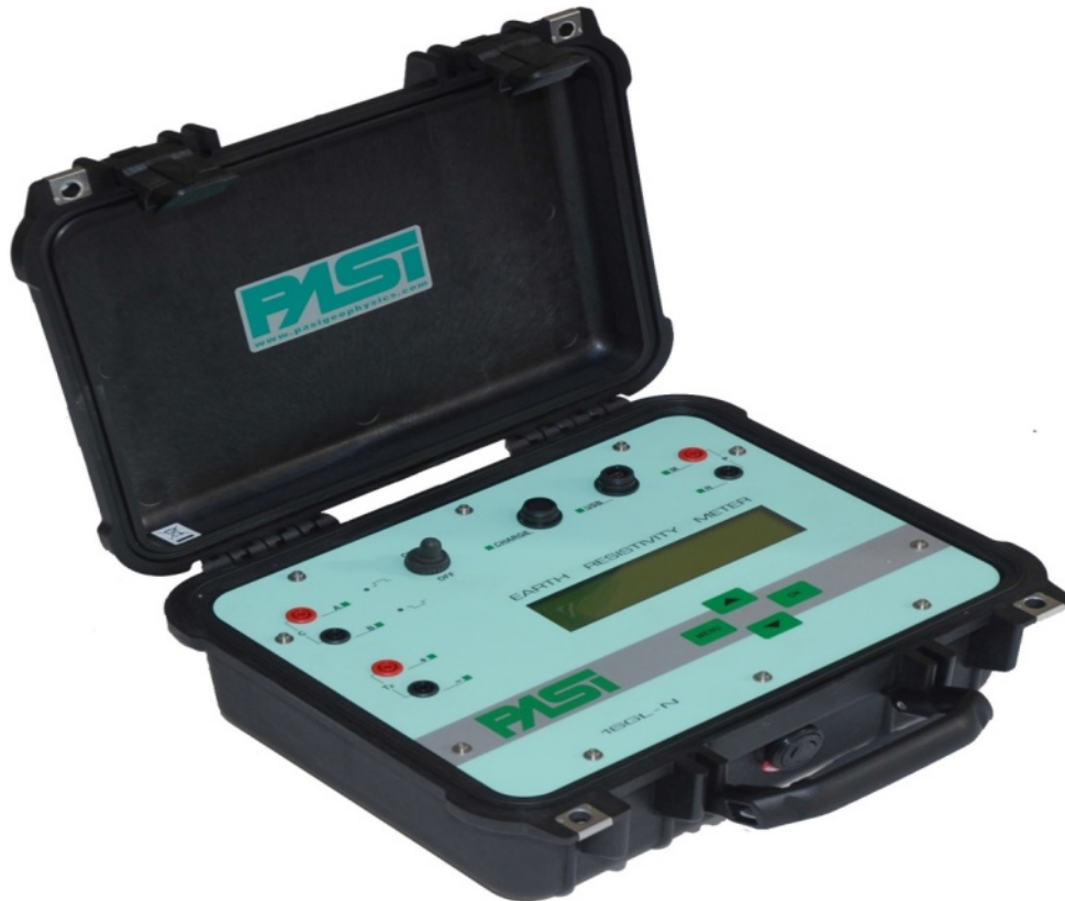
Plate 1: PASI earth resistivity meter: P100-2N; 16GL terrameter
