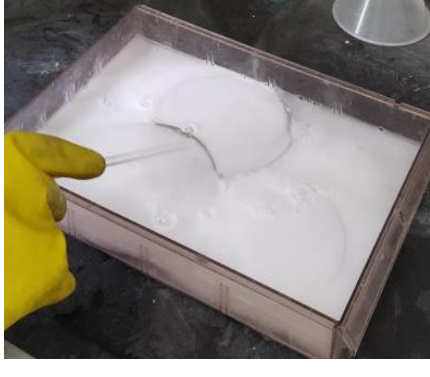
Figure 1: (a) Representation of fiber metal laminates (FMLs) (b) cutting of metal layers by wire cut machine (c) Alkaline washing of metal layers
