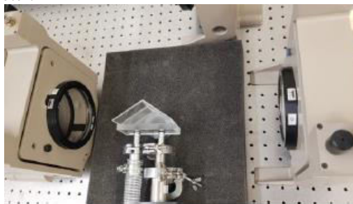
Fig. 6. Prism refractometer setup in Zygo flatness interferometer
