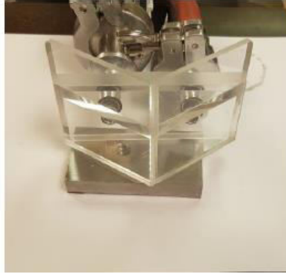
Fig. 4. Prism refractometer setup on a translation stage
