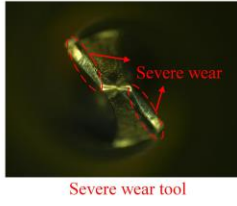
Fig. 10 (a) flank wear with different degrees of drilling tools; (b) The spectrums of the vibration data corresponding to (a)
