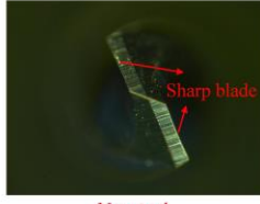
(a) Drilling tool condition
