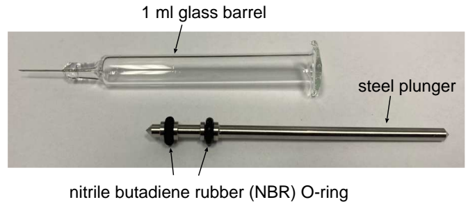
FIG. 1. A syringe used in the present experiments consisting of a 1 ml glass barrel and a steel plunger with rubber O-rings. The O-rings are sandblasted to give well defined random surface roughness.
