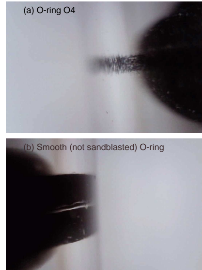
FIG. 27. The contact region between (a) the sandblasted O-ring O4 and the glass barrel, and (b) a not sandblasted (smooth) O-ring and the glass barrel. Note the incomplete contact in (a) and the apparent complete contact for the smooth O-ring in (b), except for a strip (white line) in the middle of the contact due to extra material (flash) formed at the parting lines in the mold (the flash disappear upon sandblasting).
