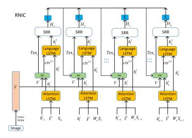
Fig. 2: The overall architecture of RNIC
