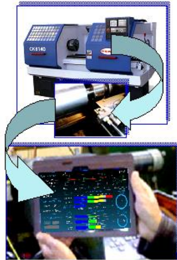
Figure 3. Automated monitoring of the technical conditions of the lathe.
