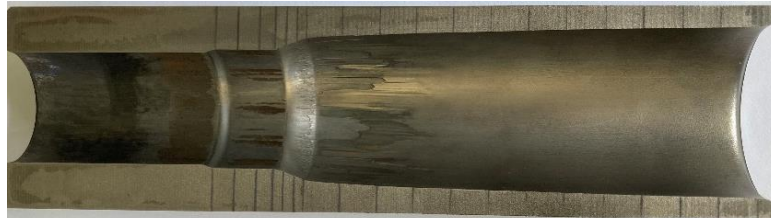
c) Machining sample of inverted cone 3° cathode after optimized
