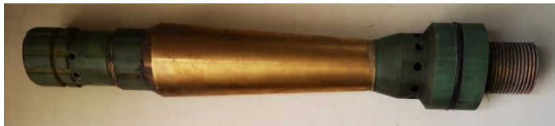
b) Inverted cone cathode after optimizing the profile
