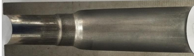
b) Machining sample of inverted cone 2° cathode after optimized
