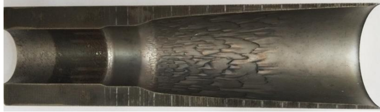
a) Machining sample of normal cone cathode with equal gap
