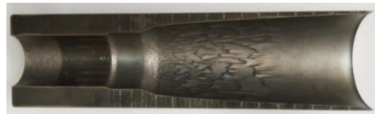
Fig.2 Sample processed with equal gap cathode
